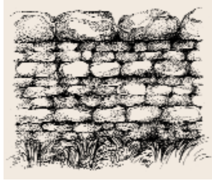
Double dry stone wall
